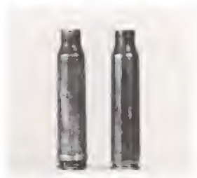
Figure 69: Centerfire Case Failure Probably Caused by a Soft Case Head
